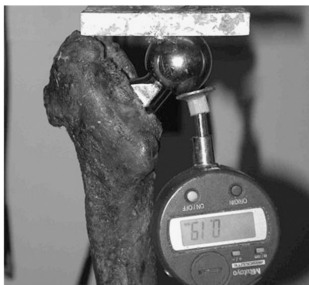
Figure 5 Evaluation of stem subsidence during cyclic axial loading.
